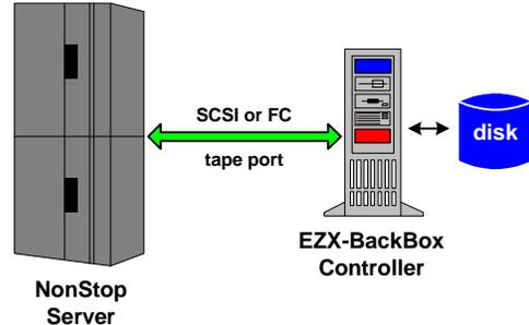
The Guardian tape I/O process is unaware that it is not driving a tape machine. Rather, the EZX-BackBox Controller emulates any one of the native tape devices used on NonStop servers. It accepts tape write commands and writes the data to disk instead of tape. It can also accept tape read commands and read data from disk, passing it to the tape process just as if it had come from tape.
