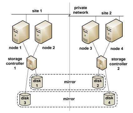
Replication may either be software-based at the host level or hardware-based at the SAN controller level. However, if SAN block replication is used, it must be guaranteed that the order of writes is preserved to maintain target database consistency.
