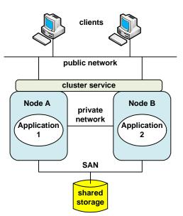
network (SAN). The cluster service is the software that programmatically connects the nodes in the cluster and provides a single-system view to the clients that are using the cluster.
