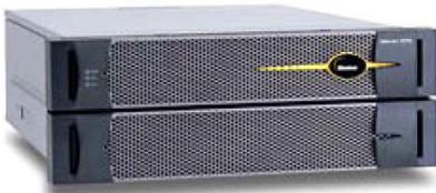
The high availability obtained by the Stratus ftServer product line is achieved by running all applications on dual processors that are lockstepped at the memory-access level. The dual physical processors appear to the outside world as a single logical processor.
