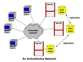
Another advantage of active/active systems is that the systems do not have to be identical. They can even be from different manufacturers. In an active/passive environment, the production and backup systems typically have to be identical. This can be a problem to maintain and leads to many failover faults in these architectures.
