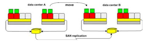
Both of these architectures achieve significantly higher availability than disaster-recovery architectures without the cost of maintaining an idle backup data center or one that is running deferrable workloads. Production workloads can be operating at all data centers.
