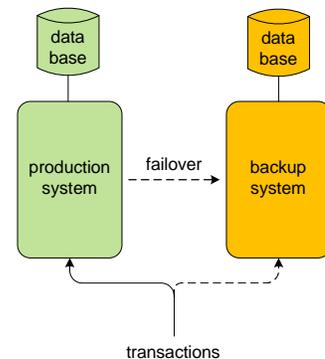
There are several architectures in which a backup system can be deployed. One architecture is to use a cold standby. In this case, the backup system may be processing some other low-priority application. When it is called upon to take over production, applications must be loaded, the database synchronized, and the network switched to route transactions to it. This process may take hours, especially if the database must be loaded from tape.
