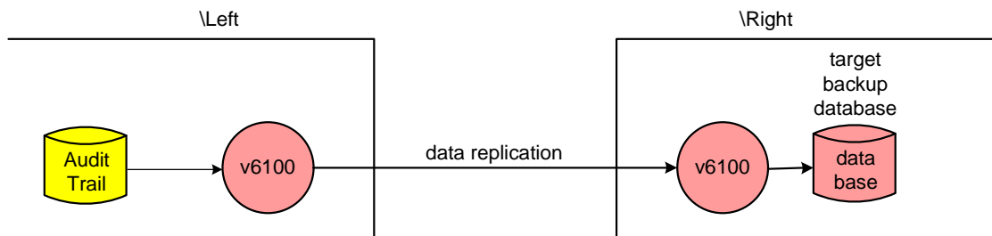
Figure 3: Replicating Data from a Source Database to a Target Database
