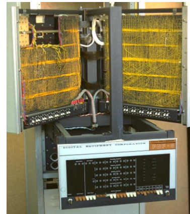
The Wire-wrapped Backplane
